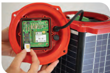
GSM module, SIM card & electronic hardware
